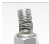
Galvanic corrosion causes TPMS failures.
