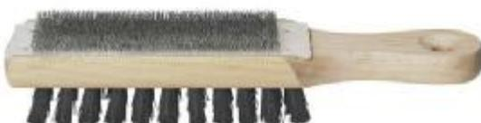
The Lutz® No. 20 Combination File Card & Brush combines the functionality and cleaning power of short steel bristles with a softer, longer bristle brush ideally suited for removing filings on finer cut files. The brush can also be used to clean saws and drill bits. A must for any shop! Overall length is 9-1/4". Packed in boxes of 6. Net Weight is 4-1/2 lbs.
