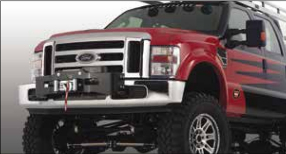
Gen II Trans4mer mounting kit, brackets, and 16.5ti winch
