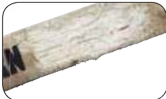
Red warning marker is encased in the strap to indicate damaged webbing
