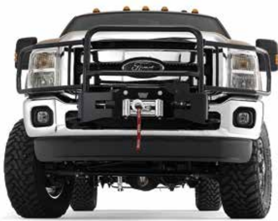
2011-15 Ford Super Duty equipped with WARN Gen II Trans4mer Mounting Kit, Grille Guard Tube (tall version), Headlamp Guards, and Light Bar
