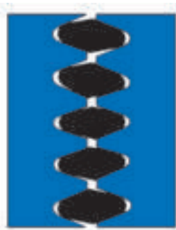
Compensation effect corrects angle and pitch error
